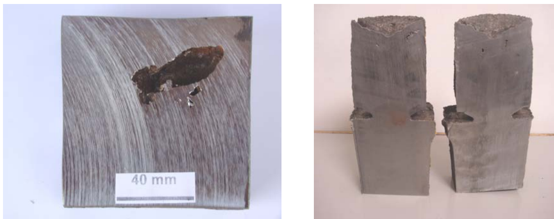
Figure 1. (A) Section of a cube made from steel without a riser; (B) same piece from Figure 1 (A) with a riser.
