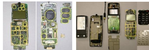
Figure 1. Disassembled components of a cell phone
